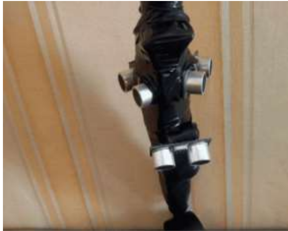
Figure 5. Ultrasonic Sensor Unit Section on the Smart Stick
