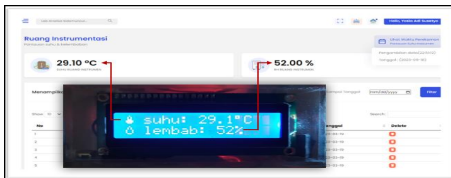
Figure 6. The IoT hardware for monitoring temperature and humidity, along with its dashboard (the name of the observation Room is written in Indonesian as Ruang Instrumentasi, i.e., Room of Instrumentation; suhu means temperature, and lembab means humidity).
