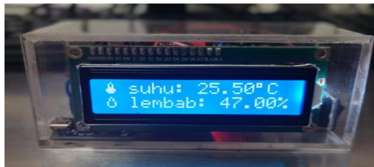
Figure 2b. IoT hygrothermometer device assembly results
