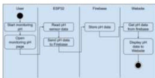
Figure 5. Activity Diagram pH Sensor
